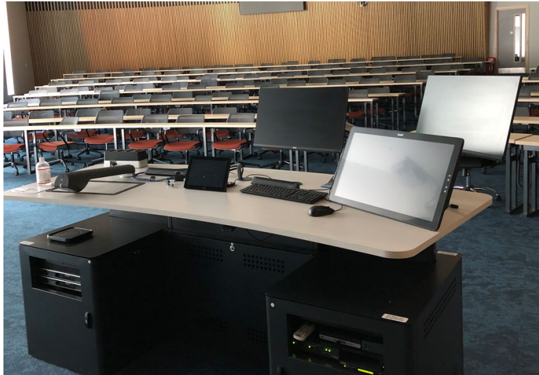
Figure 9. Lecture hall with media podium. Devices from left to right: document camera, control panel, screen 1, interactive touch panel for writing, and screen 2. (University of Glasgow).
