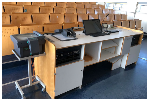
Figure 10. Podium with document camera, touch screen for drawings, and touch panels for controlling the sources. (University Halle).
